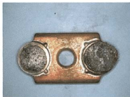
Picture 5 : relay R2-63 A1 contacts.
