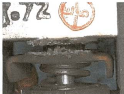
Picture 6: relay return spring
