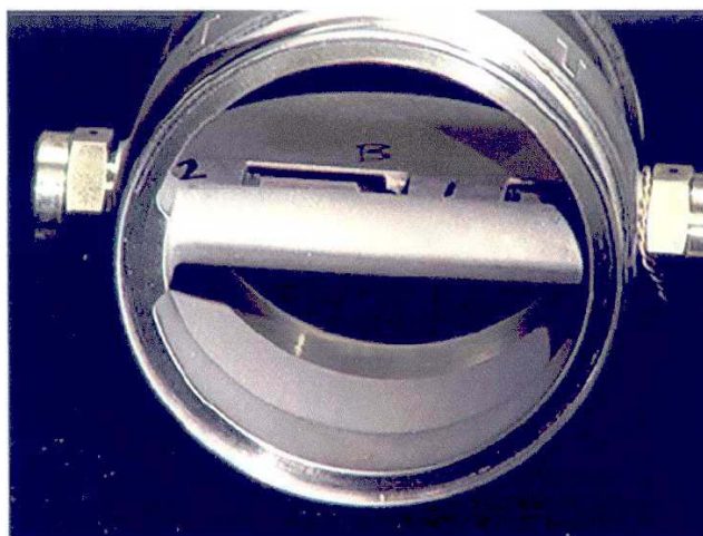
P/N 3202222-1 bleed air check valve.
