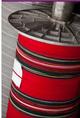
The warping is the warp preparation operation (the longitudinal threads in a shuttle fabric) and consists in transferring the yarn, contained in the reels, on the beam to be loaded behind the loom ready for weaving. The purpose of the warping is to assemble a certain number of warp threads on a single beam. The operation is performed on machines called warpers.
