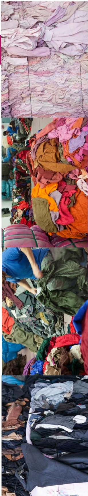
In the plant **specialized** it is carried out the lining, the selection and the classification. These operation, following an ancient tradition, are totally manual : a specialized selector, once the bale containing the various by-products has been opened, he divides the parts by type, color, fiber quality, fineness and fabric quality
