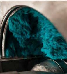
The **WASHER-SHREDDING**, it is the machine that performs the washing and shredding operations at the same time and is made up of a closed loop channel where rags, previously cut, are immersed in the water that leads them towards the working heads
